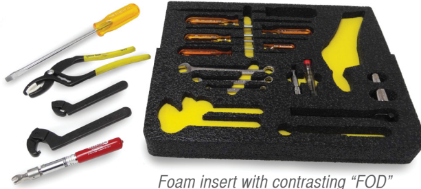
Foam insert with contrasting "FOD" foam for easy tool identification.
